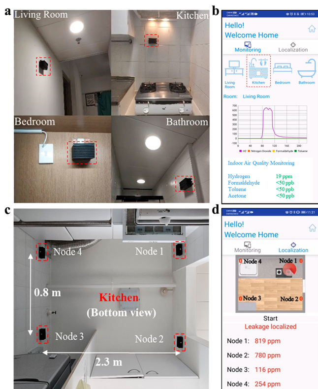
Figure 5. Smart home demonstration. (a) SINGOR systems deployed in the living room, kitchen, bedroom, and bathroom, respectively. (b) Cross-room real-time gas monitoring with the mobile app. (c) Four SINGOR systems deployed at the corners of the kitchen (bottom view). (d) Gas leakage localization with red circle flashing shown in the mobile app.
